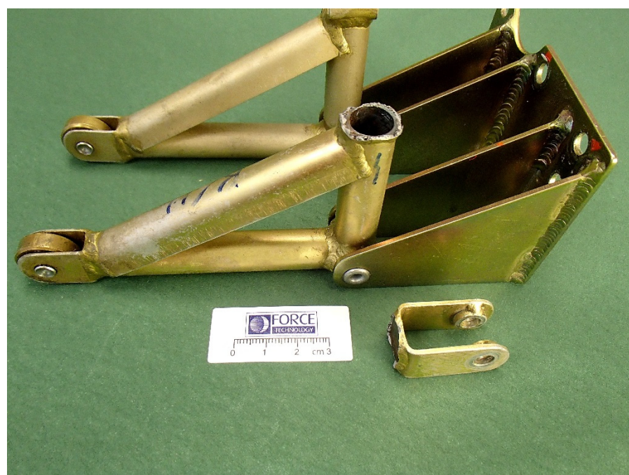
Figure 2 The left wing fractured bell crank as received.
