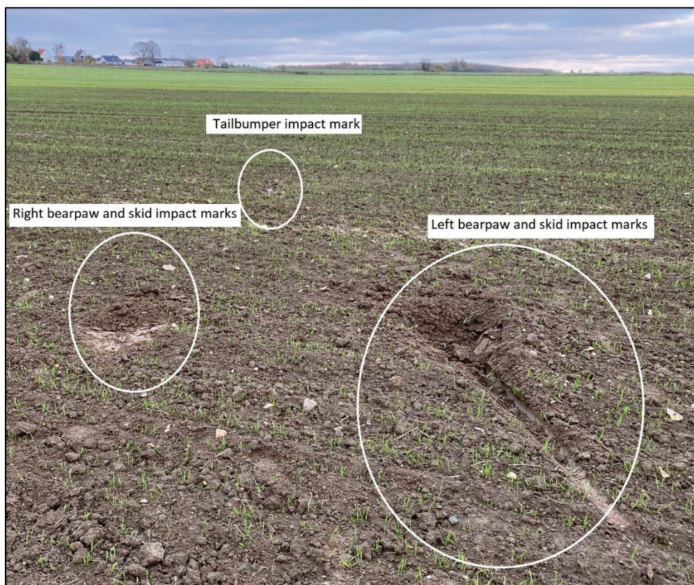
Picture no. 7 - The picture is seen from the opposite direction of the flight path, and shows the impact marks of the tail bumper, the right bearpaw and skid, and the left bearpaw and skid.
