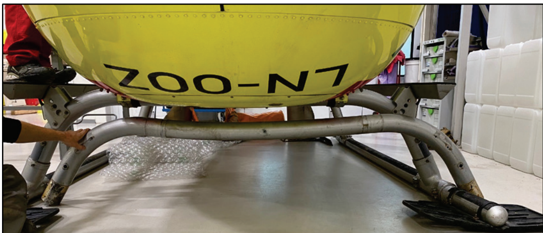
Picture no. 3 – Removed damaged aft crossbeam compared to new installed.
