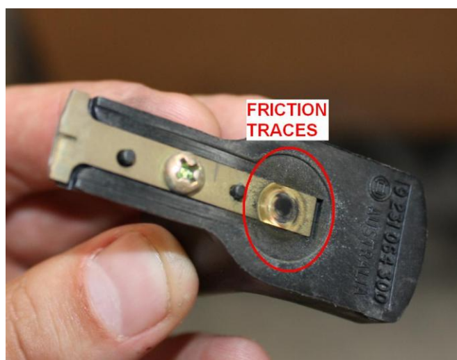
Figure 5: Friction traces on a practically new rotor
