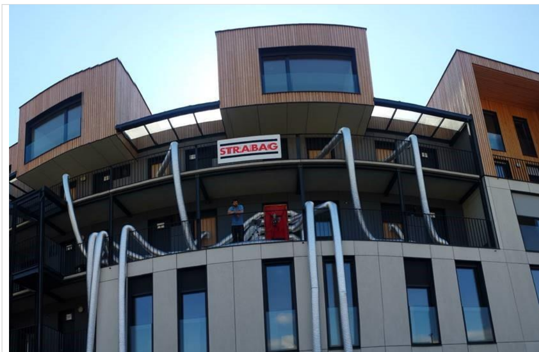
Figure 2. Airtightness quality control – Blower door tests for apartments and for the entire building were done in several stages during the construction of the building F3 Brdo, Ljubljana – a NZEB demonstration project of the Housing Fund of the Republic of Slovenia (2016) (Source: GI ZRMK, Photo: Andraž Rakušček).
